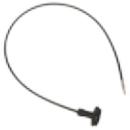
When it is necessary to make luminance measurements of objects that are inaccessible to traditional line of sight testing, the 2 foot (61 cm) 4 foot (122 cm) or 10 foot (3.05 m) long Fiber Probe provides the capability. Simply place the 0.125 in. (3.185 mm) clear aperture tip flush on the target. This accessory is available for the PR-524 only.
